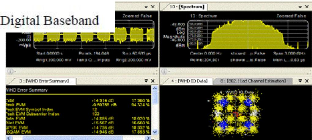
Fig. 9 Measured constellations after demodulation in the HRP2 mode (OFDM-16QAM modulation) with Agilent tools.
