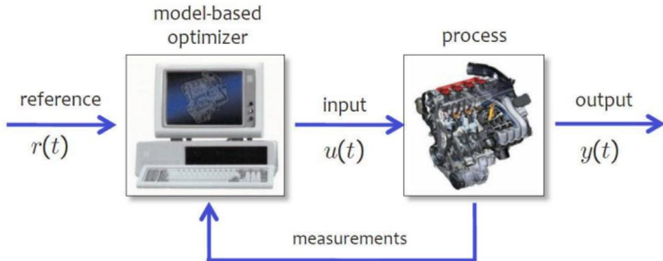
A **model** of the process is used to **predict** the future evolution of the process to optimize the **control** signal
